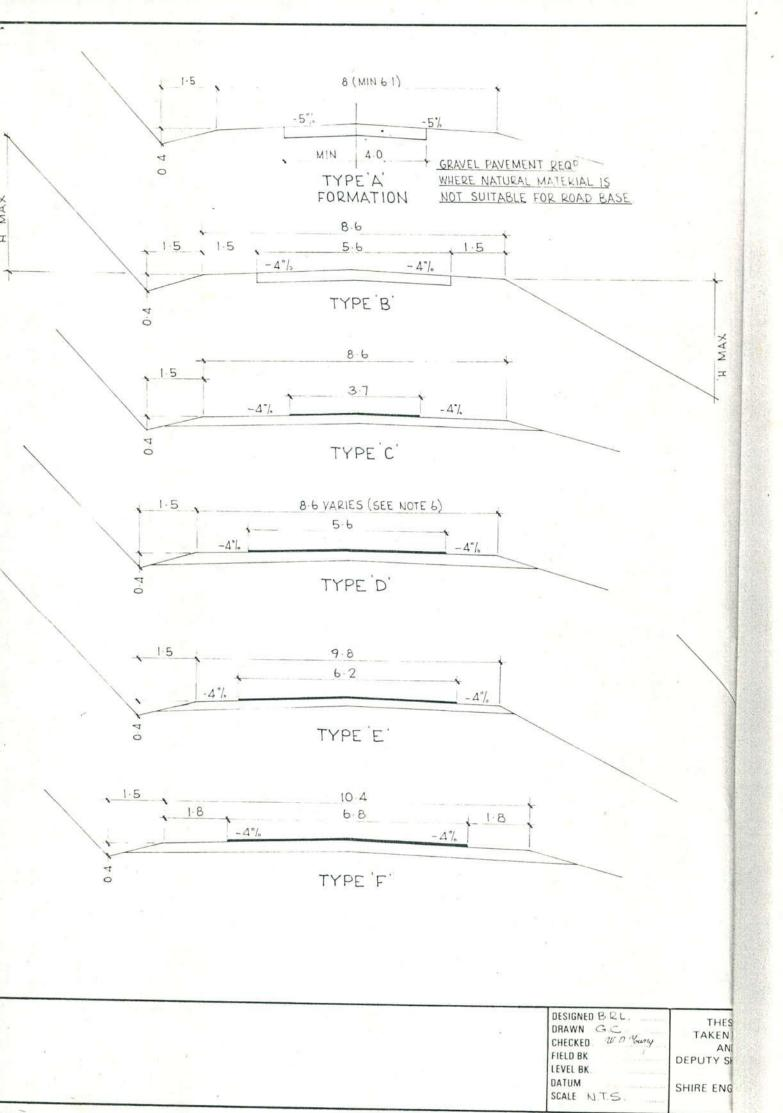
1) DESIGN STANDARDS :- DESIGN PERIOD IS YEARS LAADT. 300 100 140 1100 2200 =60 km/hr CUT FILL 2) BATTER SLOPES :- DRIFT SAND 5:1 5:1 3:1 SAND 3:1 CLAY, LOAM OR GRAVEL 1.5:1 WHERE H MAX < 1 SHALE OR OTHER MATERIAL SUBJECT 1 :1 SLOPE NOT TO TO RAPID WEATHERING. EXCEED 4:1 ROCK WITH CLAY SEAMS N.A. 0.75:1
